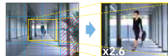
Areas with swaying trees or flickering light, etc. can be eliminated to avoid false alarms. Surveillance of the detected object can be conducted at a zoom magnification of x1.0, x1.4, x2.0 or x2.6.
