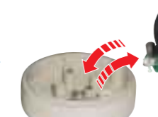
Attach the camera unit to the bottom cover mounted at the surveillance point (ceiling or wall).
