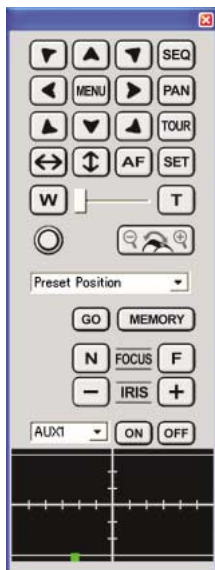
Operation panel for speed dome cameras
