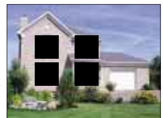
Areas with swaying trees or flickering light, etc. can be eliminated to avoid false alarms. Surveillance of the detected object can be conducted at a zoom magnification of x1.0, x1.4, x2.0 or x2.6.
